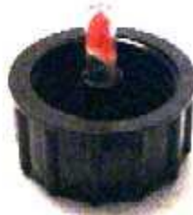
Orange wax in a sealed glass cylinder (WAPI) fits into the cap enclosure. The wax melts at a specified temperature to indicate the start of the pasteurization process.
