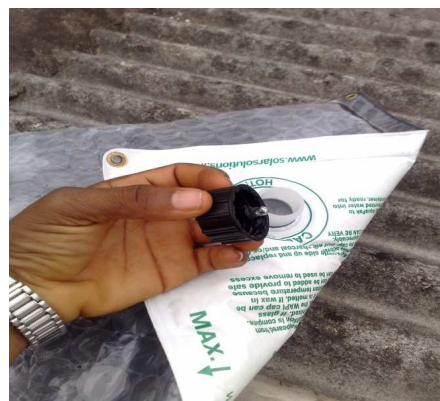
Checking if the orange indicator has disappeared
